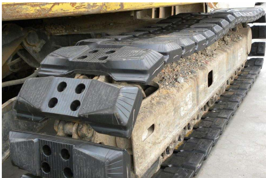
Fig 2. Example of rubber tracks on an excavator
